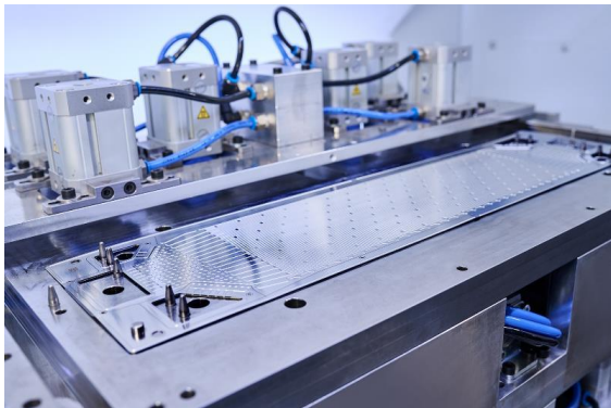
Metallic bipolar plates are a key element of fuel cell stacks. (Photo: Schaeffler)
